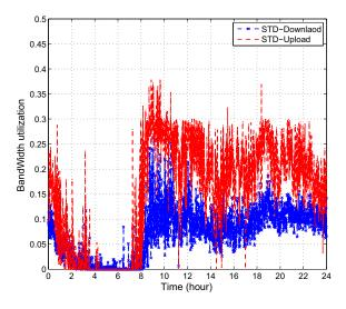
Fig. 2. Bandwidth utilization in STD.
